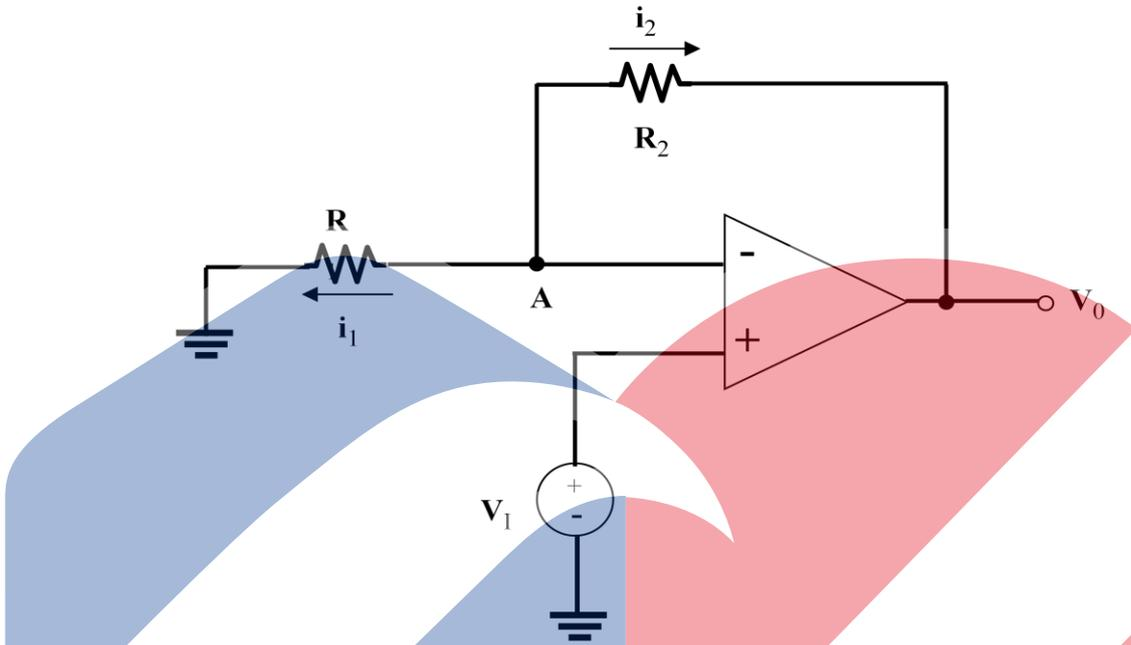
∴ Virtual ground  $\rightarrow v_{(+)} = v_{(-)}$  ,  $v_{(-)} = v_1$
